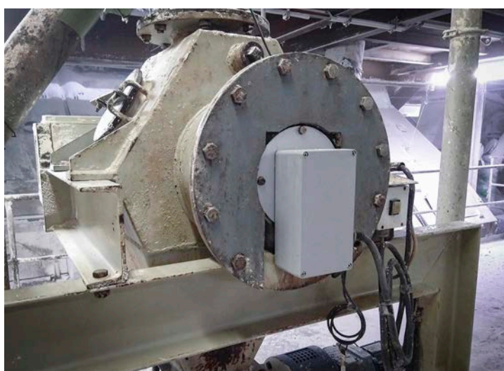
Figure 4. Potassium analyser monitors the potassium concentration after electrostatic separation.
