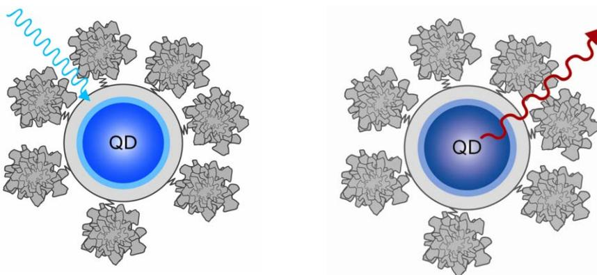
**Figure 1:** Structure of a Qdot<sup>®</sup> nanocrystal in excitation and emission state. The layers represent the distinct structural elements (core, shell and polymer coating) and are drawn roughly to scale. To the surface of the Qdot<sup>®</sup>s proteins are attached.
