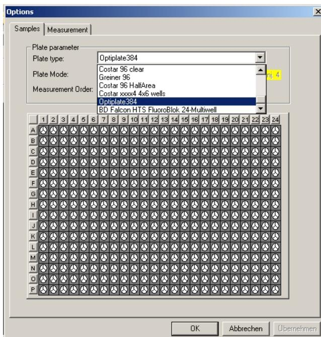
Fig.3: Selection of microplates in the Options/Read/Settings dialogue
