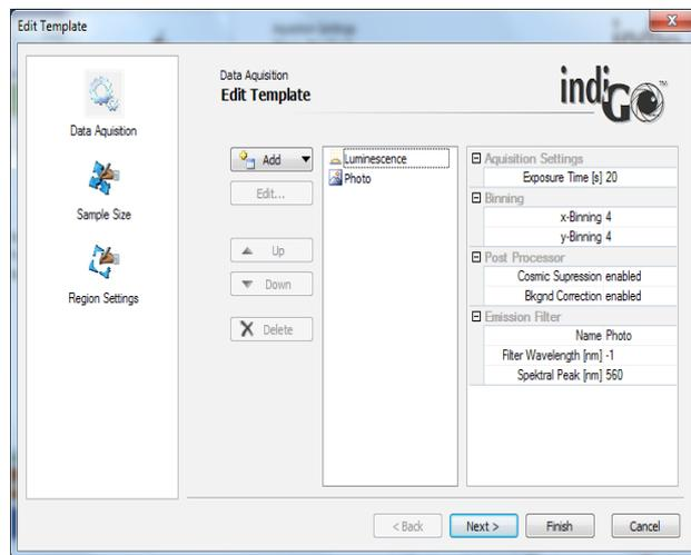
**Figure 2:** Instrument Settings in indiGO™ software: Template for delayed fluorescence measurement with defined settings.
