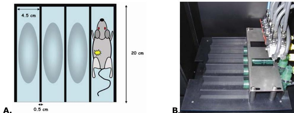
**Figure 3:** NightOWL NC 100 mice holder. Schematic view (A) of the mice holder was made by INSERM U 540, Montpellier, France and the realization of the final product was achieved by BERTHOLD TECHNOLOGIES engineers (B).
